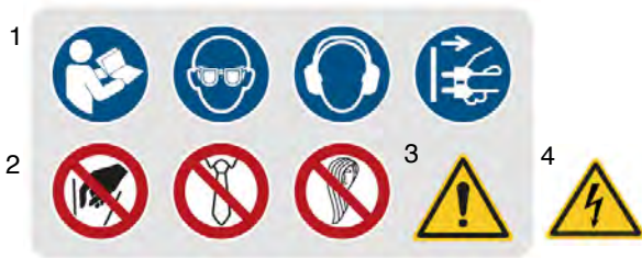
Fig. 1: 1 Mandatory sign (observe instructions for use / wear eye protection / wear ear protection / disconnect the plug) | 2 Prohibition sign (do not reach into machine / operation with loose clothing prohibited / operation with long hair prohibited) | 3 General warning sign | 4 Danger high voltage
