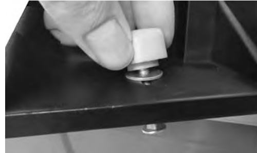
Fig. 8: Installing the spindle fence
