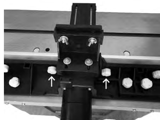
Fig. 10: Installing the spindle fence
