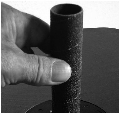
Fig. 8: Place grinding sleeve on sanding roller
