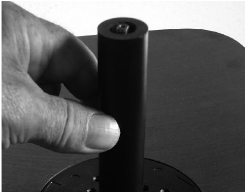
Fig. 7: Put on the sanding roller
