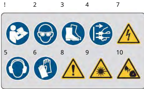
Fig. 1: Safety markings 1-6 Mandatory signs: Follow instructions for use, use eye protection, use foot protection, unplug, use hearing protection, use hand protection | 7-10 warning signs: Warning of dangerous electrical voltage, general warning sign, warning of laser beams, warning of danger from rotating saw blade
