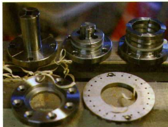
Testing Frans found that his Viper2 is about 0.2mm off centre (left), as are many of his chucks. The chuck has a good set of accessories available
