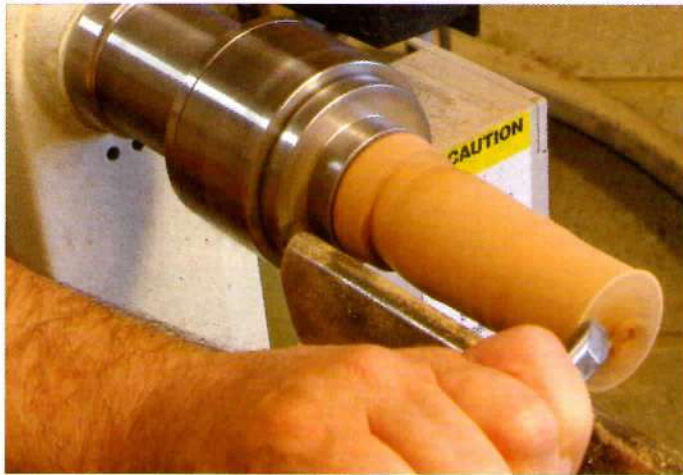
End-grain Parting across the end-grain on a spindle like this is a good test of a chuck's hold. The Viper2 performed well
