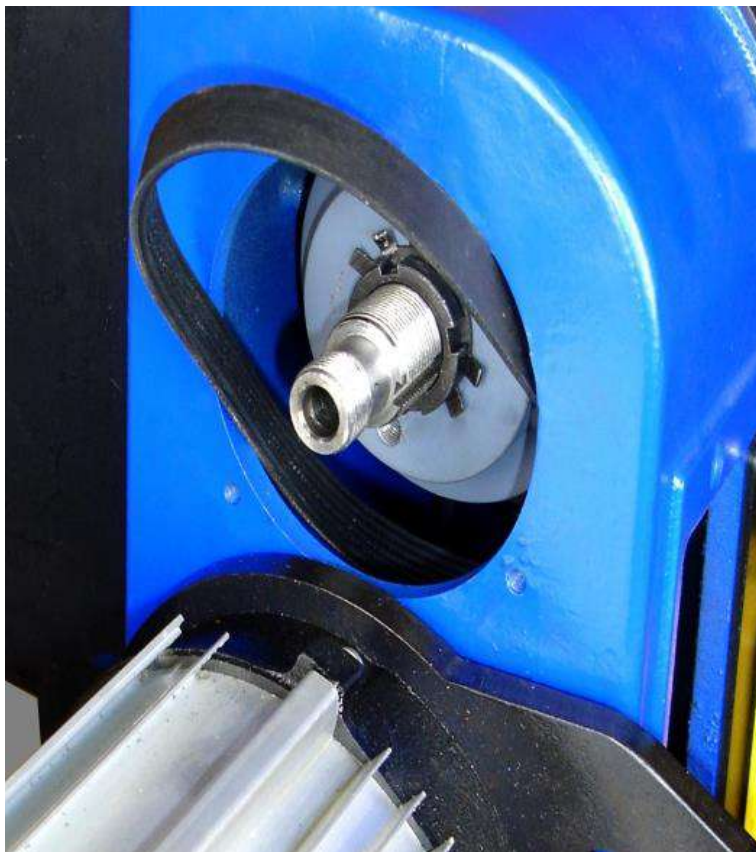
Remove Cover Plate Loosen Grub Screws Unscrew Knob
