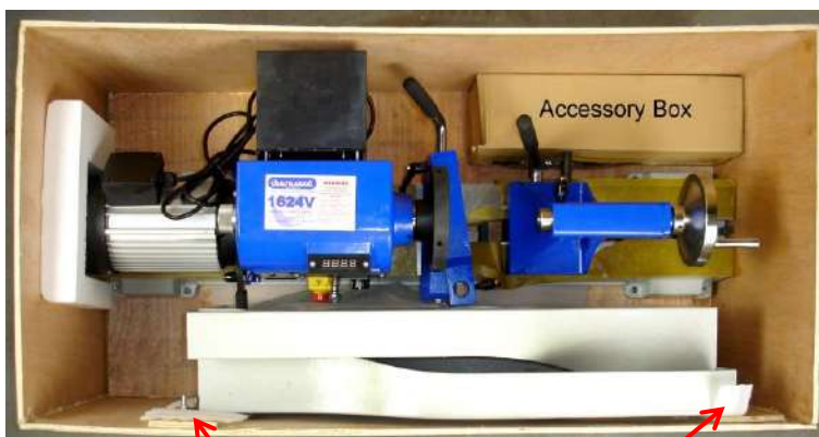
Bolts securing legs to side of crate
