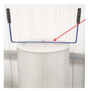
When fitting the CF2024 Cartridge filters to the W792 or W792/3 twin bag dust extractors the paddle handle must be fitted on top of the cartridge as shown in the image opposite. This will allow for both paddles to be able to turn a full rotation.
