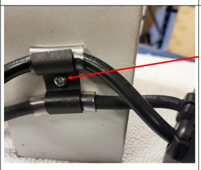
Use a cross head screw driver to remove the cable clamp.
