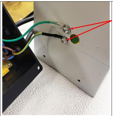
Use a cross head screw driver to remove the 2 earth cables.
