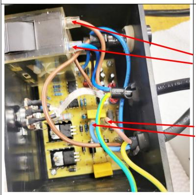
Use a pair of fine nose pliers to pull away 2 wires from the IN side of the switch.
