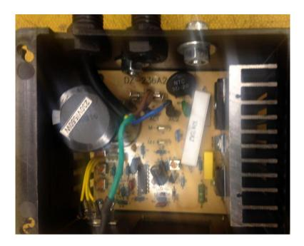
8) Pass the cable from the motor through the lower gland in the new control box and connect to the circuit board – the brown wire to the terminal marked M+ and the blue wire to the terminal marked M -. If the motor runs in reverse when started for the first time, these connections should be reversed.
