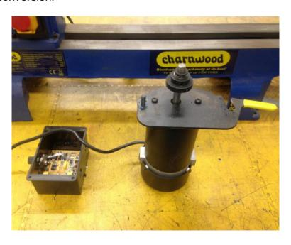
2) If the motor is being replaced, remove that too.
