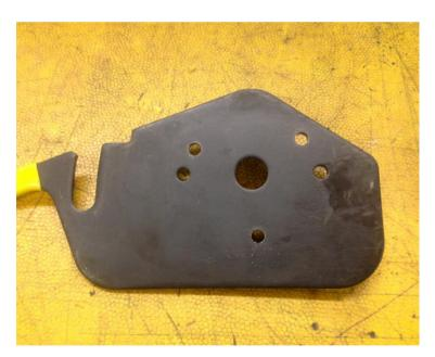
5) Mount the motor on the plate with three M6 x 15mm bolts and washers (we can supply these bolts – please ask when ordering the motor). Ensure that the motor cable is pointing to the rear of the lathe and that the motor spindle clears the hole in the centre of the mounting plate.
