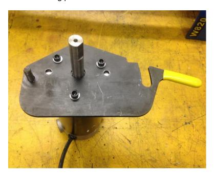
6) Fit the replacement pulley to the motor shaft, ensuring that it is the correct way around.
