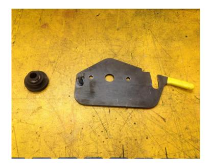
4) Mark the motor mounting plate with the position of holes corresponding to the three threaded holes in the end of the new motor. Drill three 7mm diameter holes at these points.
