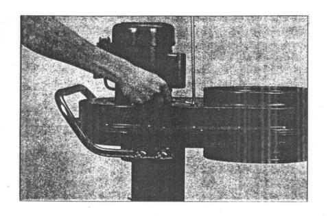
ATTACH THE UPPER BAG SUPPORT TO THE COLLECTOR BODY USING WASHER AND NUT TIGHTEN ALL FASTEN-ERS SECURELY. FIG. 5
