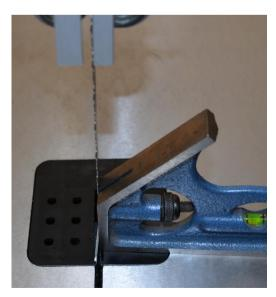
Apply a little tension to the blade and use a set square to position the table at right angles to it.
