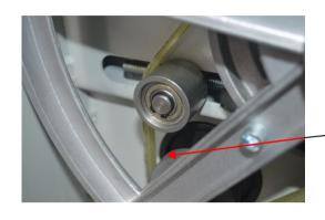
Release the belt tension by turning the tension control handle on the front of the lower housing. Move the belt from the larger pulley to the smaller one and then from the smaller to the larger on the other pair. Always have drive belt on one large and one small pulley.
