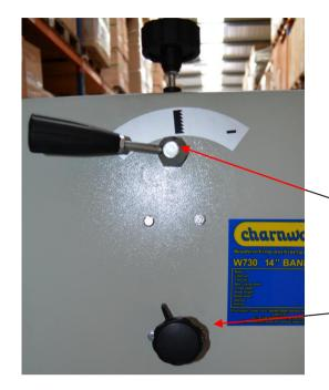
Quick blade tensioner (shown in tight position). Looking from the front, turn in an anticlockwise direction to slacken
