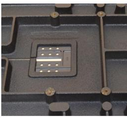
Place the table in position on the trunnion and fix it with the four bolts M8
