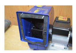
Stand the machine on its castors, place two 6mm hex head bolts through the top holes in the collector body inlet and slip the rubber gasket over them.
