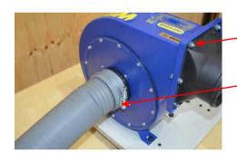
Tighten all 6 nuts on the adapter plate.
