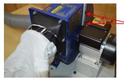
Take two hex head bolts, fit a spring washer and a flat washer over them, then use them to fix the carrying handle to the side of the fan housing.
