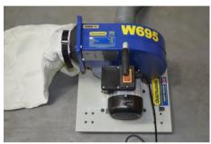
Fit the dust collection bag over the round outlet and secure it in place with the built in strap.
