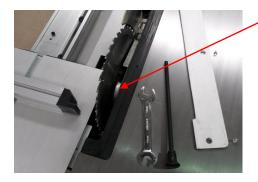
By hand, rotate the blade until the hole in the collar on the right hand side of the blade can be accessed.
