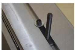
Loosen the nuts on the Tee bolts allowing them to lift enough to slide the head into the slot on the underside of the sliding beam assembly.
