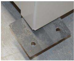
You will have to remove this fixing plate from one corner. It is secured with a cap head bolt, which can be undone with an 8mm Allen key.
