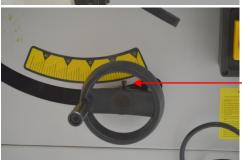
Place one hand wheel on the spindle protruding from the front of the saw.
