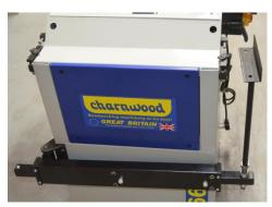
Insert the support arm into the hinged arm, as shown. You may feel a slight resistance as it engages with the internal bearings.
