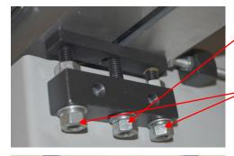
Tighten the Tee bolt nuts.
