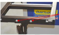
Support the sliding table with your hand and position the bracket at the top of the support arm underneath, fixing it with the four bolts that you have just removed. Tighten the two ratchet levers.
