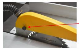
Raise the blade, loosen the nut and bolt through the crown guard and fit it over the riving knife.
