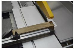
An alternative configuration is available for the sliding table. The fence can be assembled onto the front of the frame, so that the work piece is loaded against the back edge of the fence and then fed onto the blade. Using this configuration, the crosscut capacity is reduced, however some people to prefer to work this way.
