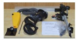
Open the blue access panel and retrieve the items shown in the picture above. You should find two hand wheels, a crown guard with extractor hose, a complete mitre fence, a hose support and a bag of fittings.
