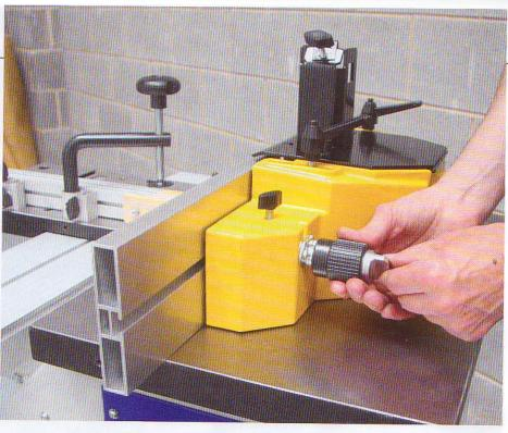
Fiddly The fence and quarding on the spindle moulder take a little getting used to, but nothing practice won't overcome, except that there's too much yellow paint on the main guard fixing slots. The sliding carriage bar (right) is relatively easy to adjust, though you have to bend pretty low to change the speeds on the spindle (right)
