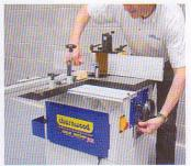
Adjustments The bar for the sliding carriage is easier to adjust than on some saws because the fettling can be done with the bar in place, which isn't always the case. The mitre fence on both the spindle and saw take a bit of getting used to, and may need a bit of work to be perfectly square. Being able to use the spindle as a router table is a huge advantage
