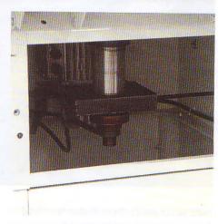
cast iron table; 1.5kw induction motor; 600x400mm table; 30mm diameter spindle; four speeds (1400, 4000, 6000, 9000rpm); 110mm vertical stroke on cutterblock; 160mm max tooling diameter; 870mm table height; 95kg; light trade rating; £599 inc.VAT; sanding drum kit £29.99; details from
