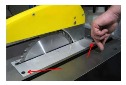
6) The two bolts holding the riving knife can now be loosened using a 13mm spanner.
