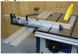
The rip fence is used to make longitudinal (with the grain) cuts. Set the fence to the required dimension using the scale provided.
