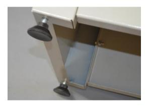
While the machine is on its side, take the four feet from the bag of parts and screw them into the four holes in the base. These feet can be adjusted by means of a spanner to level the saw table after the machine has been put into place.
