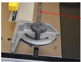
Identify the crosscut fence. Place it with the open side, face down and the plastic tip to the right. Slide the pivot block and the locking block onto the back side of the fence with the head of the bolt in the T-slot.
