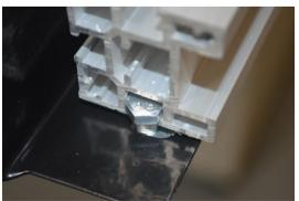
Now take the first of the extension tables, loosen the nuts and bolts and slide it onto the guide rails.
