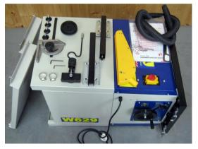
Lay the saw onto its side to remove further items which are packed inside the floor stand of the machine.
