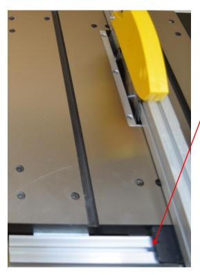
Position the rip fence parallel to and up against the saw blade.
