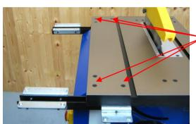
Fit the two support arms which will carry the guide rail for the sliding carriage.
