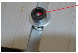
The guide rail is fitted with front and rear travel stops.
