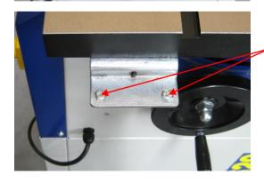
Loosen the nuts and, lifting each bolt head in turn, slide one of the 100cm long square aluminium extrusions over them.
