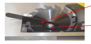
Use the special spanner supplied, lock the spindle by fitting it over the black locking washer.
