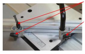
If an angle is to be cut, undo the thumb screw and ratchet lever, swing the fence to the desired angle and lock them both off.
