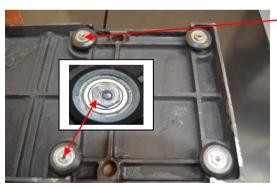
Before fitting the sliding carriage it should be noted that the two outboard bearing wheels are mounted on eccentrics.
