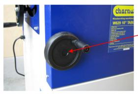
Raise the saw blade by turning the fitted hand wheel at the front of the machine clockwise.
