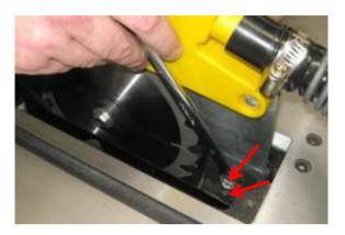
5) Raise the riving knife and crown guard assembly, so that the crown guard is situated just above the top of the saw blade. If necessary adjust the riving knife so that there is an even gap of around 5mm between the curved leading edge of the knife and the radius of the saw blade.
