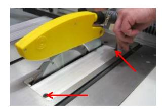
4) The two bolts holding the riving knife can now be loosened using a 13mm spanner.
