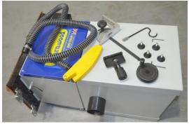
Lay the saw onto its side to remove further items which are packed inside the floor stand of the machine.
