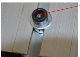
The guide rail is fitted with front and rear travel stops.
