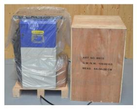
Cut the straps and remove the lid of the crate from the base.
