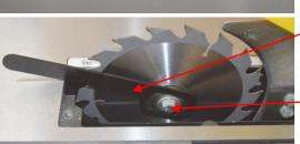
Remove the right hand table insert, using a 4mm Hex key to remove the two screws.
