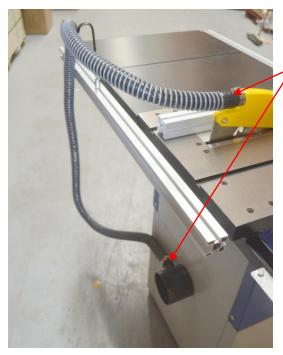
Slide the hose support clip onto the rear guide rail and lock it into place.
