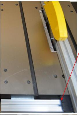
Position the rip fence parallel to and up against the saw blade.
