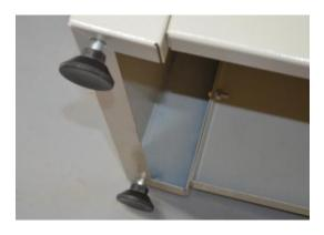
While the machine is on its side, take the four feet from the bag of parts and screw them into the four holes in the base. These feet can be adjusted by means of a spanner to level the saw table after the machine has been put into place.
