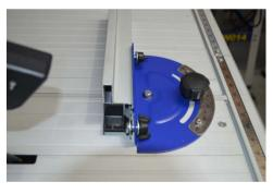
The sliding mitre fence is assembled in a similar manner, using the remaining guide bar and two short coach bolts and wing nuts.
