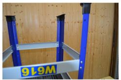
Bolt on the four lower rails, noting that the ends are angled to match the splay of the legs. Use coach bolts as before.
