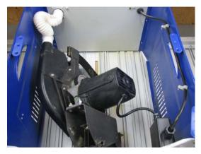
The carbon brushes must be replaced when the carbon block has less than 5mm of material remaining. Failure to replace them in time may cause damage to the motor armature, which can be expensive and difficult to replace.
