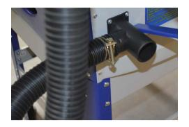
Fit the other end of the extractor hose to the side of the T connector at the back of the machine, as shown.
