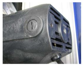
Use a flat screwdriver to remove the plastic cap.
