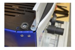
Leave all bolts finger tight until assembly of the legs is completed.
