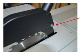
Remove the bolt and wing nut from the crown guard and fit the guard over the top of the riving knife. Replace the bolt and wing nut. Tighten them securely.
