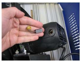
Check for wear, anything less than 5mm in length should be replaced.
