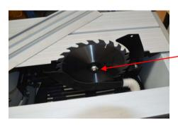
Use a 10mm spanner to hold the spindle stationary whilst using the 24mm spanner supplied, to unlock the securing nut. The blade can now be removed.
