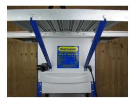
Fit the slots in the rear extension table over the heads of the bolts.
