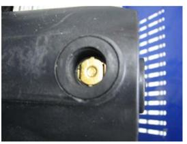
Use a small screw driver or pliers to pull out the brush.
