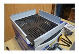
Do the same with the rails marked 'A', fitting these to the sides.
