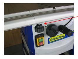
The side extensions are locked in place with the four large, black knobs which screw into the underside of the main table.
