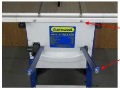
Bolt the two blue support arms to the back of the saw.
