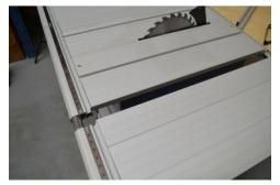
Attach the two side extension tables by pushing the round metal tubes into the corresponding holes in the end of the main table.
