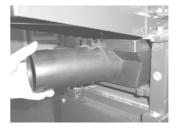
Note: unless the hood is correctly located, the planer will not work. This is not a fault – it is part of the machine's safety system.
