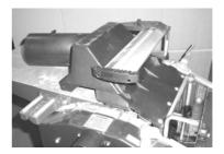
Important Safety Notice – the chip collection hood also functions as the cutter block guard when the machine is set up for thicknessing.
