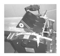
If you are using a dust extractor (this is strongly recommended), prior to securing the collection hood, place the extraction hood over it and then secure as detailed above.
