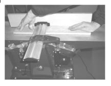
Once the face side has been satisfactorily planed, the face edge can be machined. Check that the fence is set at the required angle. Slide the guard across the table so that the work can pass between the fence and the guard and lower the latter to its minimum height. Lock the guard in place. The plastic end cap of the guard should exert slight pressure on the work.
