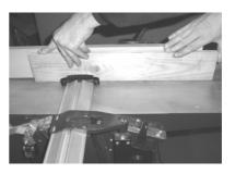
Start the machine and keeping the work firmly pressed against the fence, pass it slowly over the cutter block.
