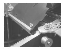
2.7 Fix fence bracket to the carrier with an 8 mm coach bolt and then fix the fence to the carrier with the two knurled nuts supplied. Note that the shorter nut is placed adjacent to the 90/45° stop adjusters.
