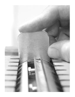
Use the 3mm Allen key supplied, adjust the projection of the knives by turning the three setting screws of the lock bar in or out as required. When the settings are correct (keep checking with the gauge) fully tighten the lock bar's hex bolts. Start with the centre bolt and work outwards.
