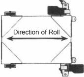
A short narrow base, such as a Morticer or Bandsaw, will benefit from this arrangement. The casters are in a wider position which reduces the amount of tilt during raising and lowering of the foot levers.
