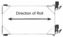
A long narrow base, such as a Lathe, will benefit from this arrangement with both foot levers on one end.
