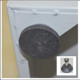
Fix the four feet to the base of floor stand, placing one washer on the threaded portion of each foot before passing it through the hole, adding the second washer and the spring washer, followed by the nut. Tighten securely.
