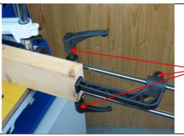
The length stop can be set to aid production runs where a series of identical components are to be produced.
