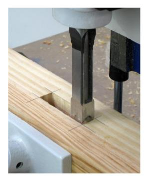
Position the table so that the chisel cuts almost its complete width. The chippings will be ejected into the space created by the previous cut. Continue moving along the mortice, cutting a series of holes, until the complete length of the mortice has been cut.
