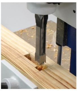
If the width of the mortice is bigger than the chisel being used, use the central hand wheel to move the table backwards and again repeat the procedure to cut another series of holes in front of the first set.
