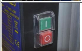
To start and stop the morticer, it is fitted with an NVR switch, located on the left hand side of the motor housing.
