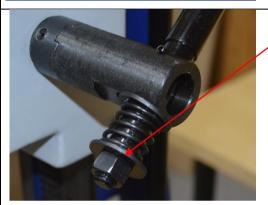
Take the handle and pass it through the hole in the shaft. Secure it with the spring, washer and nut provided.
