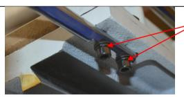
Bolt the end stop to the underside of the sliding bed, using the socket head bolts and washers provided.
