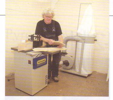
Chippings A spindle moulder produces much more chippings than a router table, but the combination of 100mm port on the fence, and the Fox extractor make it pretty much dust-free. You can buy special cutters for tenons, or just cut two rebates
