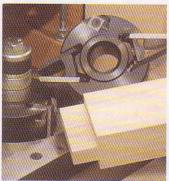
micro-adjustment on each fence, so that you can position the outfeed forward to account for what you've removed in shaping.
