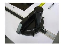
SACRIFICIAL FENCE:- The mitre fence can be enhanced by adding a longer wooden sacrificial fence to the front of the sliding fence. The sacrificial fence can run all the way up to the cutter and can be used to prevent breakout on the back edge of the work piece.
