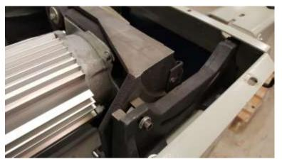
2) Cast iron trunnions: The W650 has cast iron trunnions securely held on a welded frame
