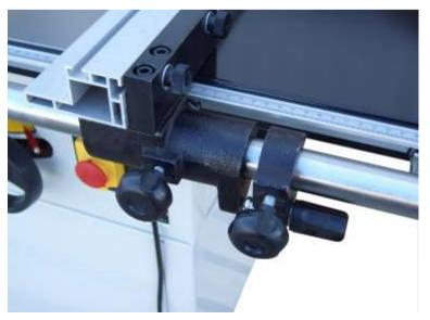
1) Rip Fence: The W650 has a more substantial rip fence design, using an industrial style polished solid steel bar. It is quicker to set and features a micro adjuster to enable fine adjustments to be made, for those times when a very accurate setting is required.
