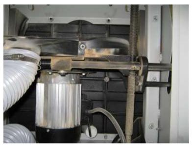
4) Heavier control bars: used to control blade height, and blade tilt
