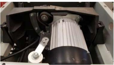
3) Cast iron motor mount: The W650 has a heavy duty mounting bracket designed for professional users
