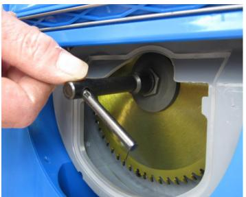
Refit the large washer, ensuring that the flat sides of the centre hole are aligned with the flat sides of the shaft.
