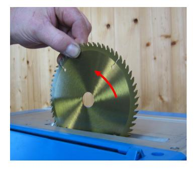
Next feed the sawblade down through the slot in the table.
