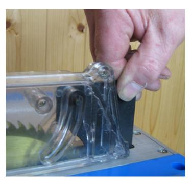
Take the blade guard and riving knife assembly. Feed the bottom end of the riving knife down into the slot, directly behind the blade. Push it down until the transparent guard sits on the surface of the table.
