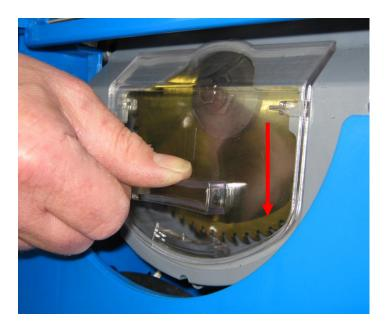
Refit the transparent cover. Push it firmly downwards to lock it into position.
