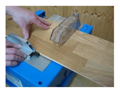
To prevent the back edge of the wood from splitting out, the fence should always be adjusted so that the tip on the right hand end of the fence is touching the blade. It is made of a soft plastic which will not damage the blade.
