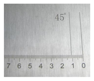
When making a rip cut at 45 degrees it is necessary to make an adjustment to the position of the rip fence, due to the altered position of the blade.
