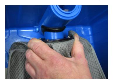
From time to time, or when you notice a decrease in the performance of the vacuum function, it is necessary to empty the dust collection bag.
