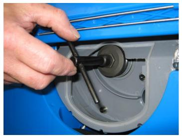
Using the spanner provided, remove the blade retaining bolt by turning it anticlockwise.
