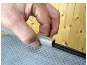
To empty the dust bag, slide the plastic sealing strip along the opening edge of the bag and empty the contents.
