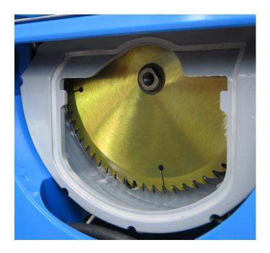
Align the sawblade so that the centre bore hole fits over the shaft.
