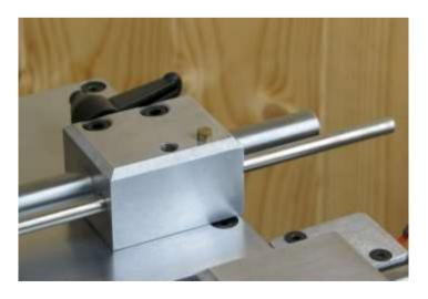
Place the Brass Nipple (S) into the threaded hole in the fence block.
