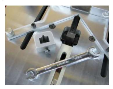
To clear a blockage; remove the cap, using a spanner. Once removed, the driver should drop back down and the jammed wedge can easily be removed.
