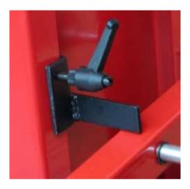
The Locking clamp can also be used to lock the footpedal half way down, This reduces the amount of travel required to insert a wedge and is speeds up the pinning operation when working with small mouldings.
