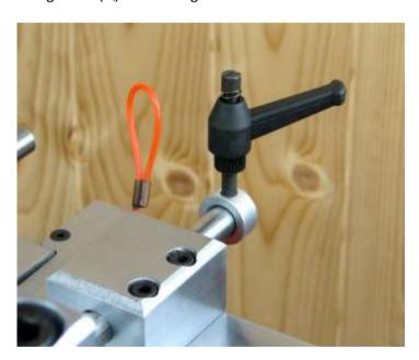
Insert the Front Stop Bar (A) into the hole in the fence block.
