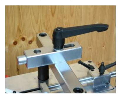
Push the adjusting button inwards and insert the vertical bar from above (C). Screw the L Shaped Pad (F) on to the end of the vertical bar.
