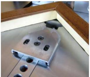
Release the foot pedal and the clamp will move forward, gripping the moulding. The tip of the clamp is designed to allow for slight variations in the moulding width.
