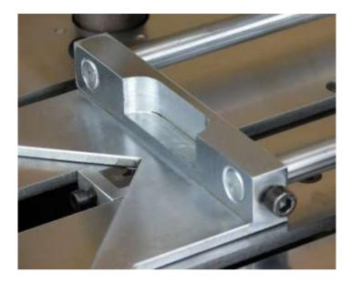
Fit the Handle and Locking Collar (Q) over the right hand fence bar.
