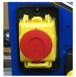
In this example we are using Switch model KJD12, manufactured by KEDU.
