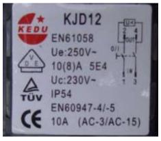
3) Make a note (or take a picture) of which colour wires attach to which terminals. The switch terminals, 4 of them in this case, are labelled 'In' and 'Out' and numbered.
