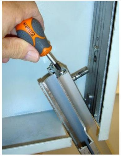
If possible, wind the shaft and pinion gear out of the top of the extrusion.
