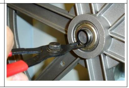
Fully remove the vertical locking and adjusting knobs taking care to retain any springs/washers fitted to the shaft.
