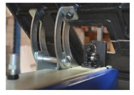
Pull the left hand edge of the table tilt trunnion upward as shown. Remove the plastic insert from the table. From the back of the bandsaw, slide the table forwards allowing the blade to pass through the slot in the table.
