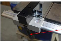
Place the rip fence on the table, with the black handle in the raised position, seat the assembly on to the guide rail.
