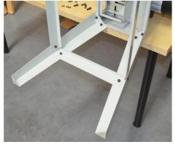
Bolt on the four leg braces, noting that the fold goes to the upper side.
