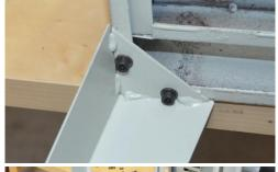
Leave all nuts and bolts finger tight until you have finished assembling the stand.
