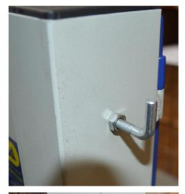
Screw a nut onto the push stick hook and screw this into the tapped hole high up on the left hand side of the saw. Lock it into position with the nut.
