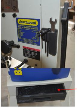
Hang the push stick on its hook and place the Allen keys and the spanner into the tool holder.
