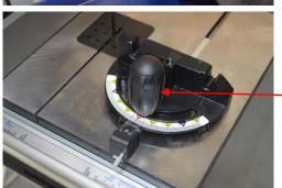
Slide the mitre fence into one of the T-slots in the table.
