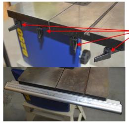
Screw the four large, plastic wing bolts into the tapped holes along the underside of the front edge of the table.
