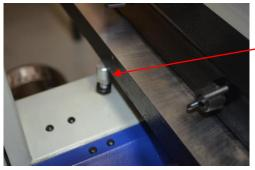
This special bolt sets the angle of the table for 90° cuts. When the edge of the table is resting on it, the blade should be perpendicular to the table top. If necessary this bolt may be loosened and an adjustment made.
