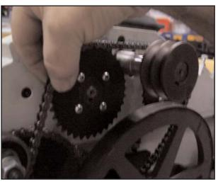
8) Lower The drive assembly to gain access to the spring adjusting nuts.
