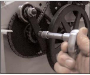
7) with the mechanism still supported by your spare hand remove the feed roller drive chains.
