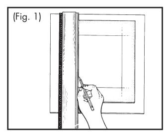
**Step 1- Mark the Mat**Using the scale, mark the back of the mat for the exact border you want. (Fig. 1)
