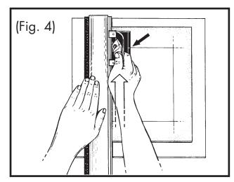
Lower the heel of your hand behind the mat cutter and push away from yourself keeping pressure constant until the indicator line lines up with the top intersecting pencil line. (Fig. 4)
