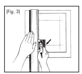
Step 3 - Cut the Mat Hold the guide rail firmly with your left hand. Place your thumb on the retractable blade holder and exert downward pressure forcing the blade into the mat. (Fig. 3)
